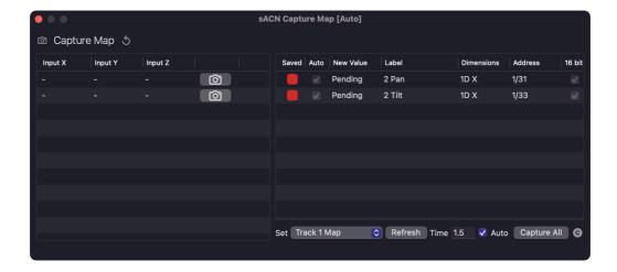
As you capture the buttons will highlight. These can be reset using the reset (rotating arrow) button top left.
