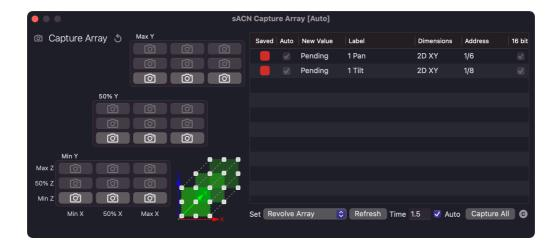
Click a capture (camera) button to communicate with the console specified in Settings to set the channels to the associated target from the selected capture set. The values are then captured, and the Conversion output value is updated. See Input/Output.
