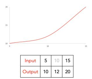
The diagrams below are illustrative of non-linear Maps. The curves illustrate how the presence of multiple points can impact the resulting output because all points are evaluated to produce a continuous curve. Note: This is provided for information only, actual output may differ.
