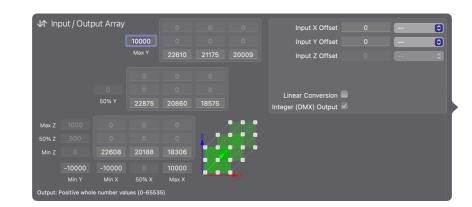
The 3x3x3 grid of output values represents 3D space, the bottom left of the 3 boxes being the near Y positions and the top right the far Y positions.
