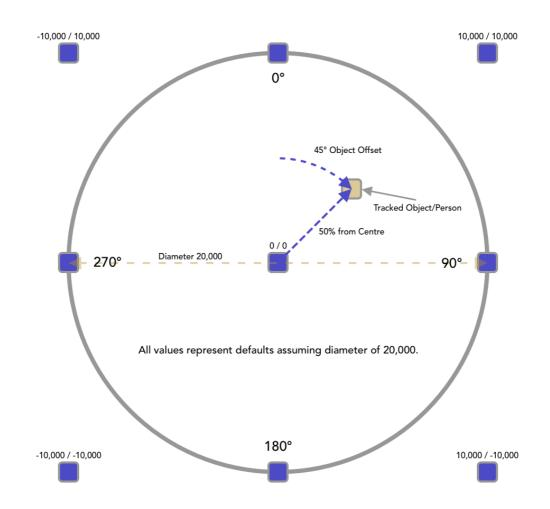
A tracked object is illustrated, showing how the Object Offset and % from Centre values are calculated.
