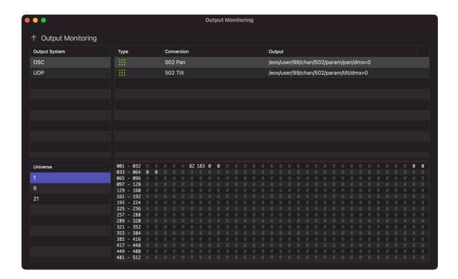
Select an Output System on the top left of the window and any outgoing conversions in that system will be displayed in the panel on the right. The traffic light output indicator on the left shows whether data output is currently enabled and the output value is displayed and updated in real time (when enabled).
