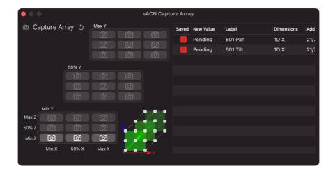
Select the Conversions you wish to update in the main window. This selection will be replicated in the sACN Capture window. Click a capture (camera) button to capture the current values and update the Conversion output value for that field. See Input/Output.
