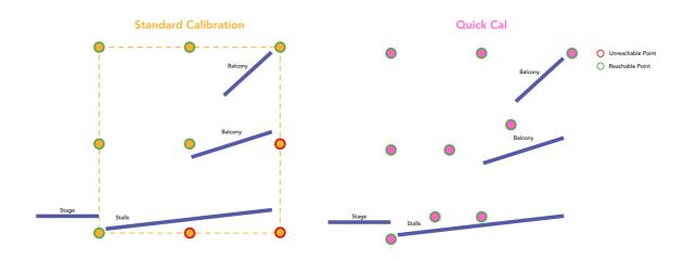
Note: The closer together the points are, the less accurate the final result will be. It is recommended to capture points at the greatest possible extents.
