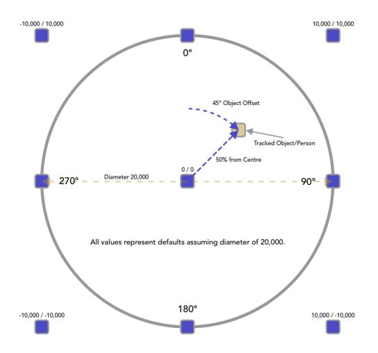
A tracked object is illustrated, showing how the Object Offset and % from Centre values are calculated.
