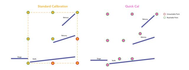
Note: The closer together the points are, the less accurate the final result will be. It is recommended to capture points at the greatest possible extents.
